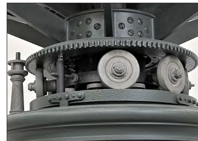
Clockwork mechanisms from the 1854 Fresnel lens.
