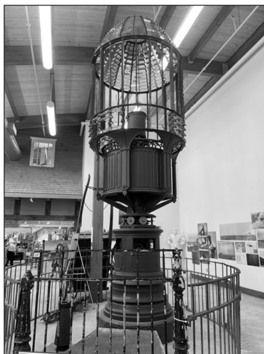
Cape Hatteras' 1854 1st Order Fresnel lens.
