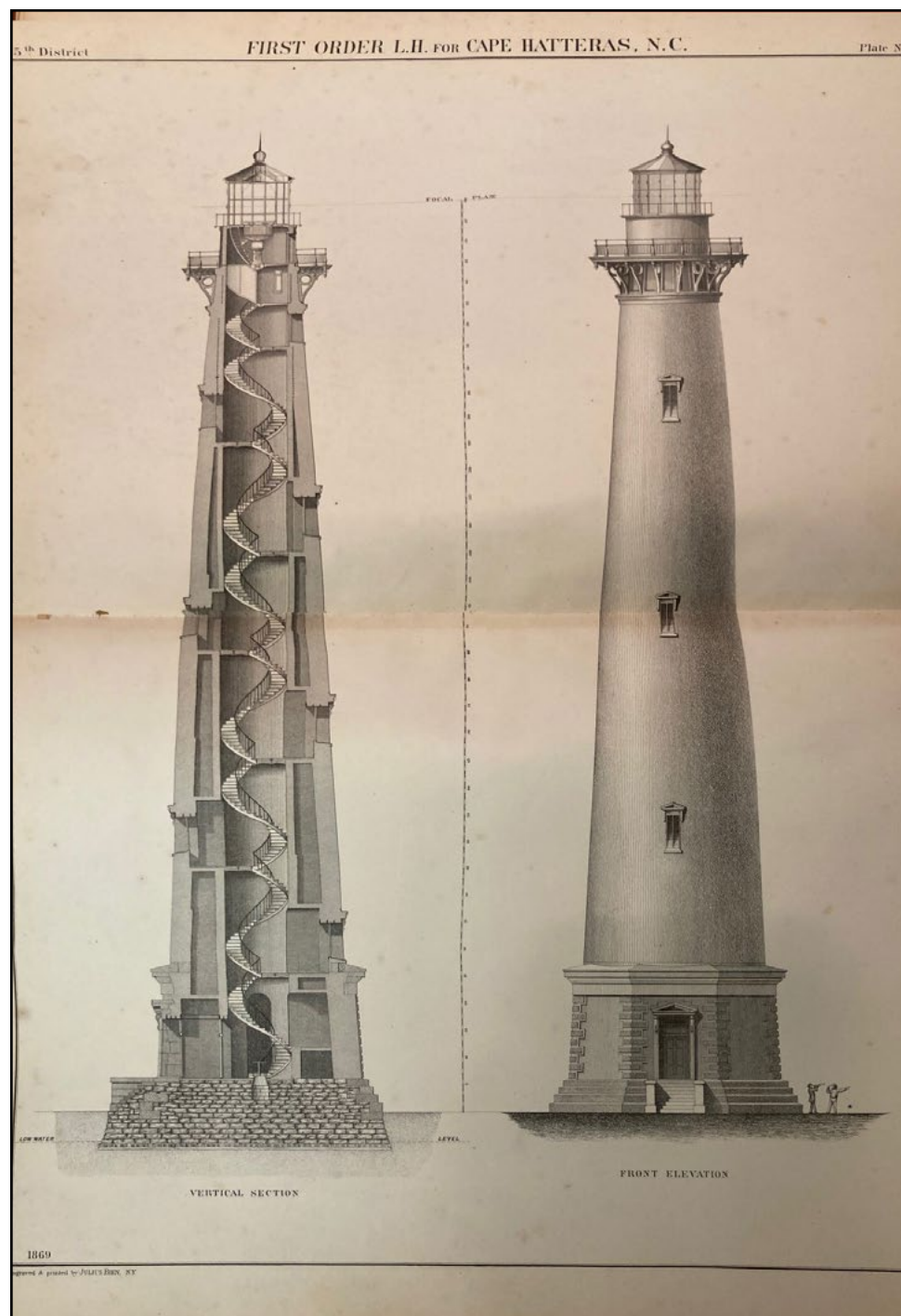
Vertical section and front elevation for First Order light house for Cape Hatteras, NC.
